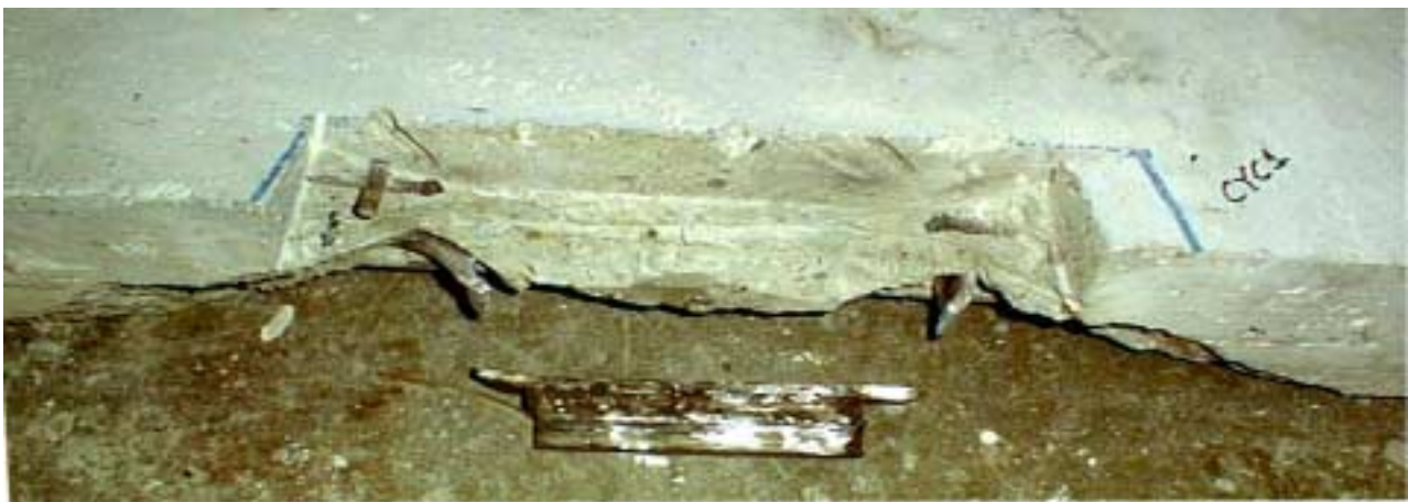
Figure 6. Condition of concrete near connector is shown after completion of cyclic test #1. Note that the topping concrete above the connector was sawn away to provide welding access to the connector
