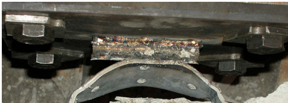
Figures 30 through 32: Typical Failure for Tension Only Test
