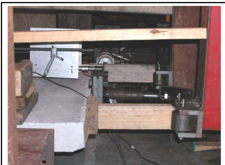
Figure 8: Side View of Tension Test Setup
